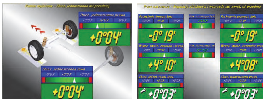
Fig.4 Toe-in adjustment and results for the wheels of the test vehicle
