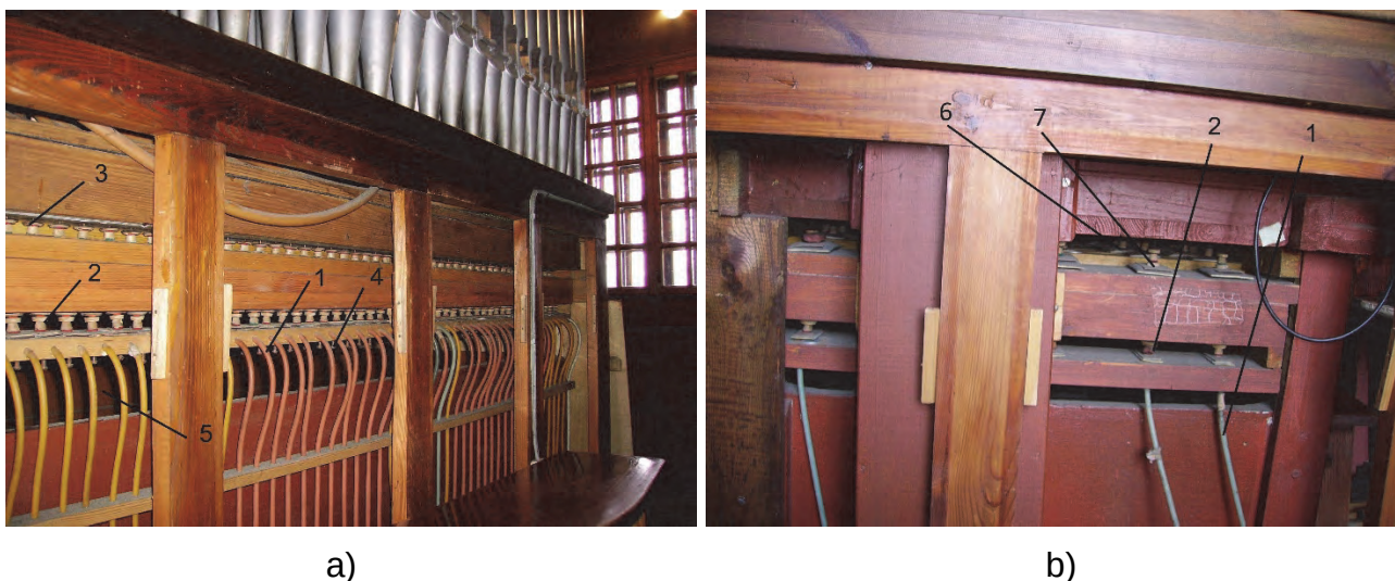
Fig.3 Pneumatic action in the organ at St. Roch's in Nowy Sącz [3] a - play action, b - stop action
