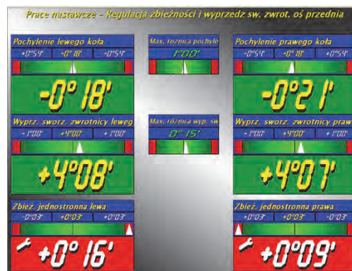
Fig.3 Results of the vehicle wheel alignment measurement
