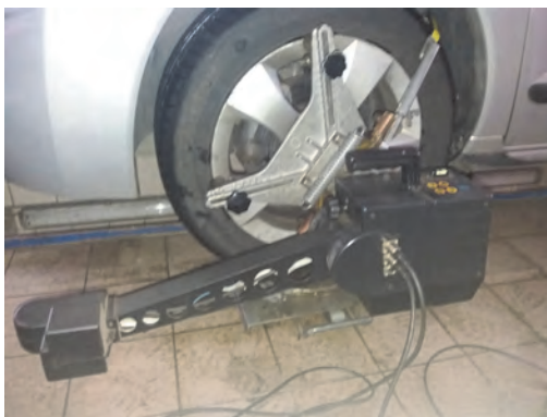
Fig.1 The vehicle on the test bench with the connected measuring head
